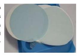
Biologically inert, NC membranes are widely used in clarification, sterilization and analytical applications. Show an exceptionally low level of extractable verses other membranes in the market.
